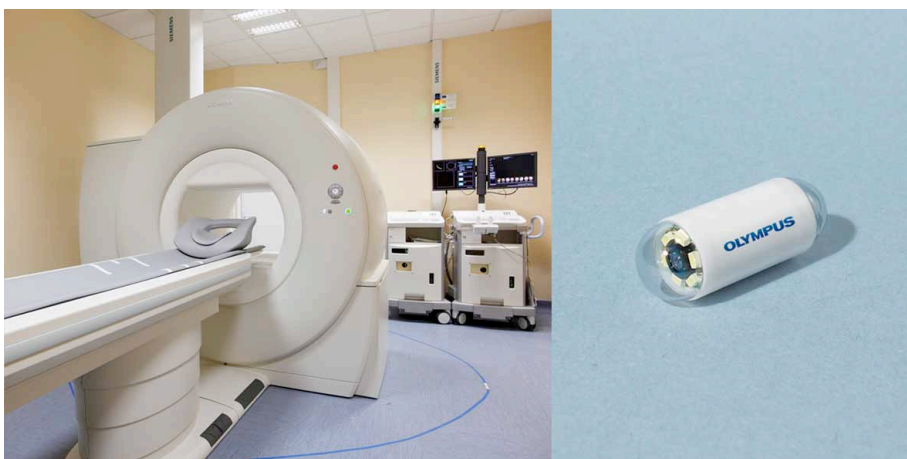
Picture: The prototype guidance magnet, image processing and guidance information system, and capsule endoscope.
